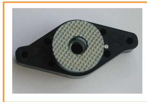
Figure 1 c. Place grinder/compressor cap onto shaft of measuring cell. Rotate clockwise. Note: Stainless steel stop pin on right-hand side of cap
