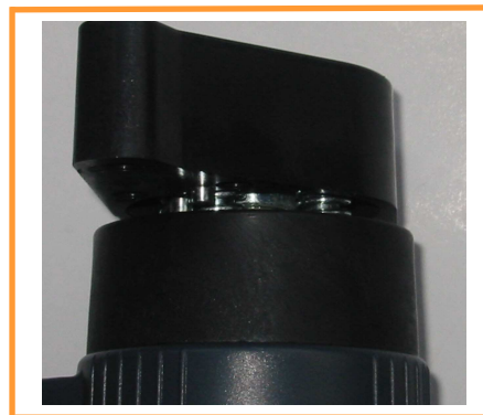
Figure 1 d. Screw down the cap clockwise until the stainless steel stop pin in the cap and measuring cell prevent further rotation.
